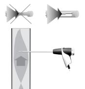
The flue gas must be able to flow freely past the thermocouple.
